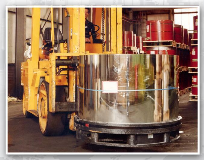
The KLP® Rollpallet® has been developed in close co-operation with Hoogovens IJmuiden (nowadays known as Corus), in the Netherlands. It was designed to improve means of transport and storage of coils with the eye to the sky. Standard sized KLP® Rollpallet® are suitable for coils with diameters ranging from 940 mm to 1760 mm diameter.
